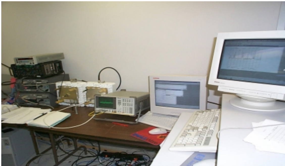
Figure 22: Test setup photo for Conducted Spurious Emission for Both Hub and Sub 38 GHz High band ODUS.
