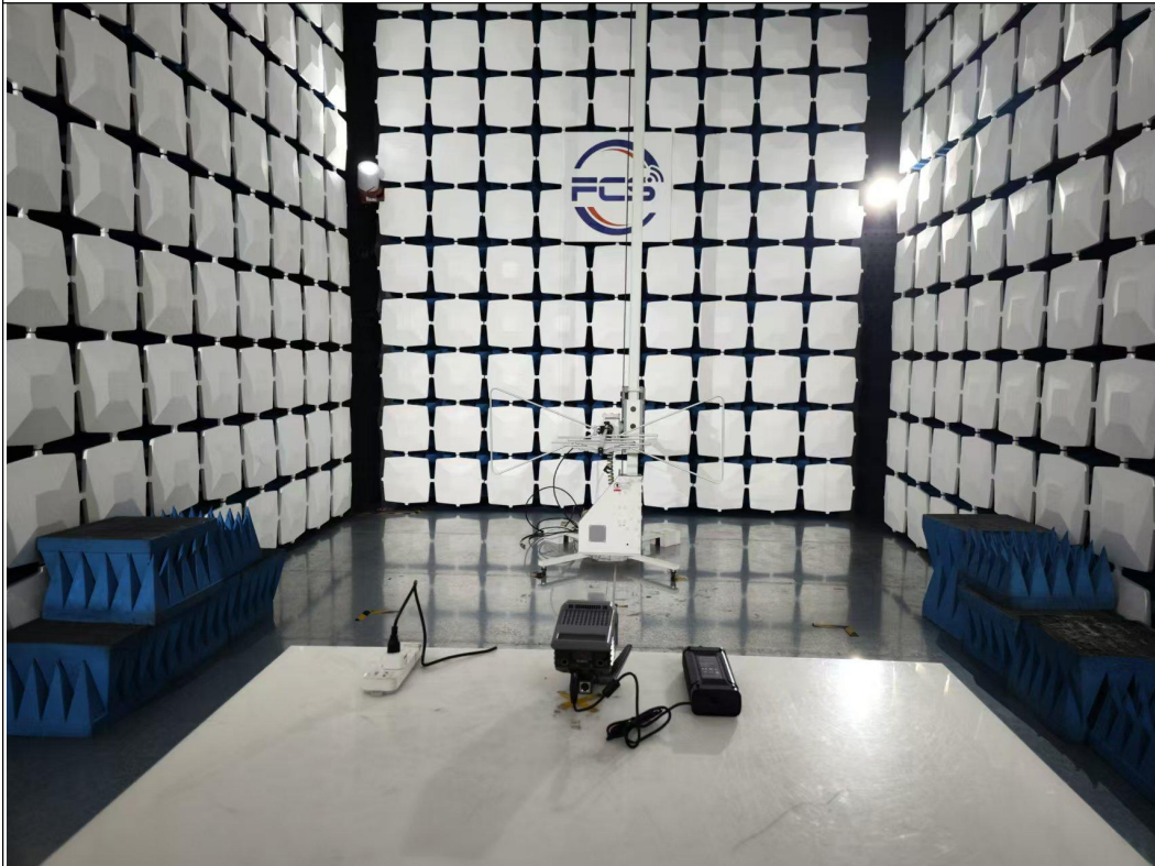
Above 1GHz for radiated emission test setup
