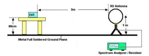
For radiated emissions from 30MHz to 1GHz
