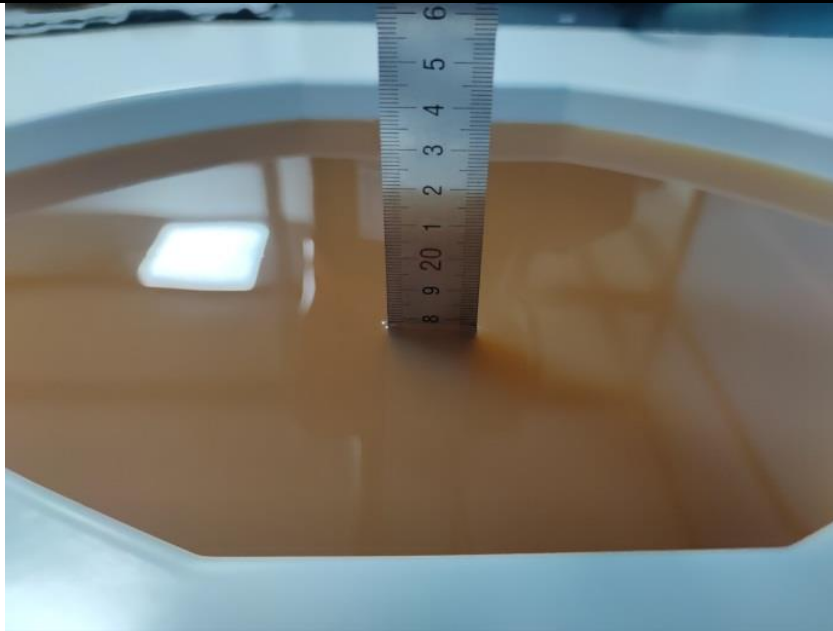
Fig. 9.1 Photo of Liquid Height for Extremity SAR (depth>15cm)
