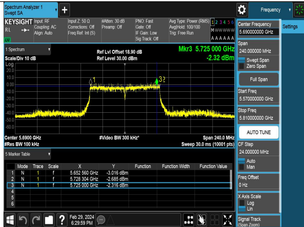
Mode:802.11ac VHT80 Frequency:5690MHz Ant:Chain0 scope:NII2C
