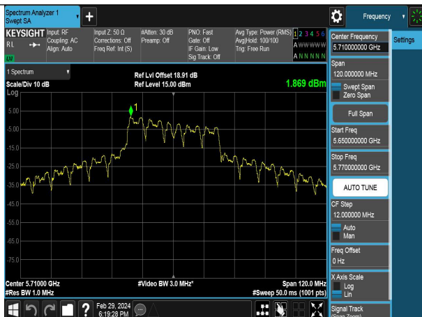
Mode:802.11ac VHT40 Frequency:5710MHz Ant:Chain0 scope:NII2C
