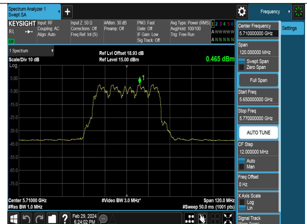
Mode:802.11ac VHT40 Frequency:5710MHz Ant:Chain1 scope:NII2C
