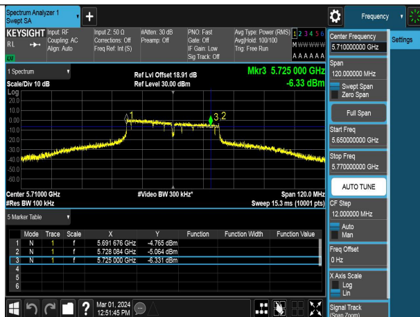
Mode:802.11ac VHT40 Frequency:5710MHz Ant:Chain0 scope:NII2C
