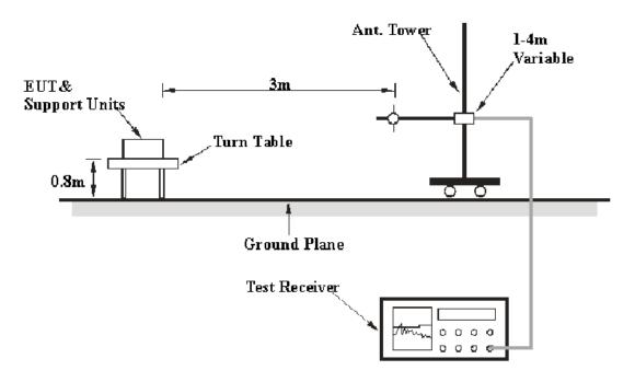
The radiated emission tests were performed in the 3 meters, using the setup accordance with the ANSI ANSI C63.10-2013. The specification used was the FCC Part 15.205 and 15.209 and 15.227 limits.
