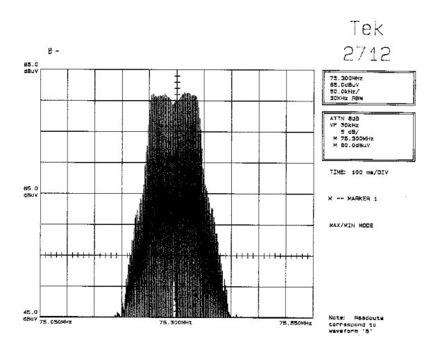
Result : The field strength of any emission within the operation band did not exceed 98 dB( $\mu$ V/m) for average value or 118 dB( $\mu$ V/m) for peak value. Refer to page 9 &12 for the recorded value for the emission at the fundamental frequency.
