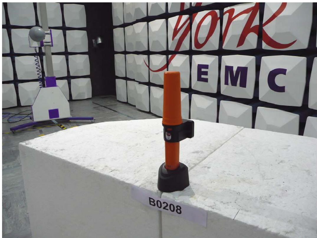
Figure 5.6.3 Radiated Emissions 1GHz to 2GHz Testing
