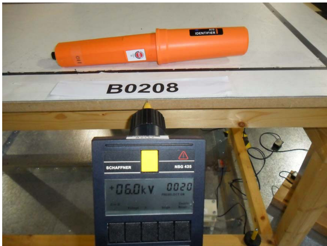
Figure 5.6.5 ESD Testing – Contact
