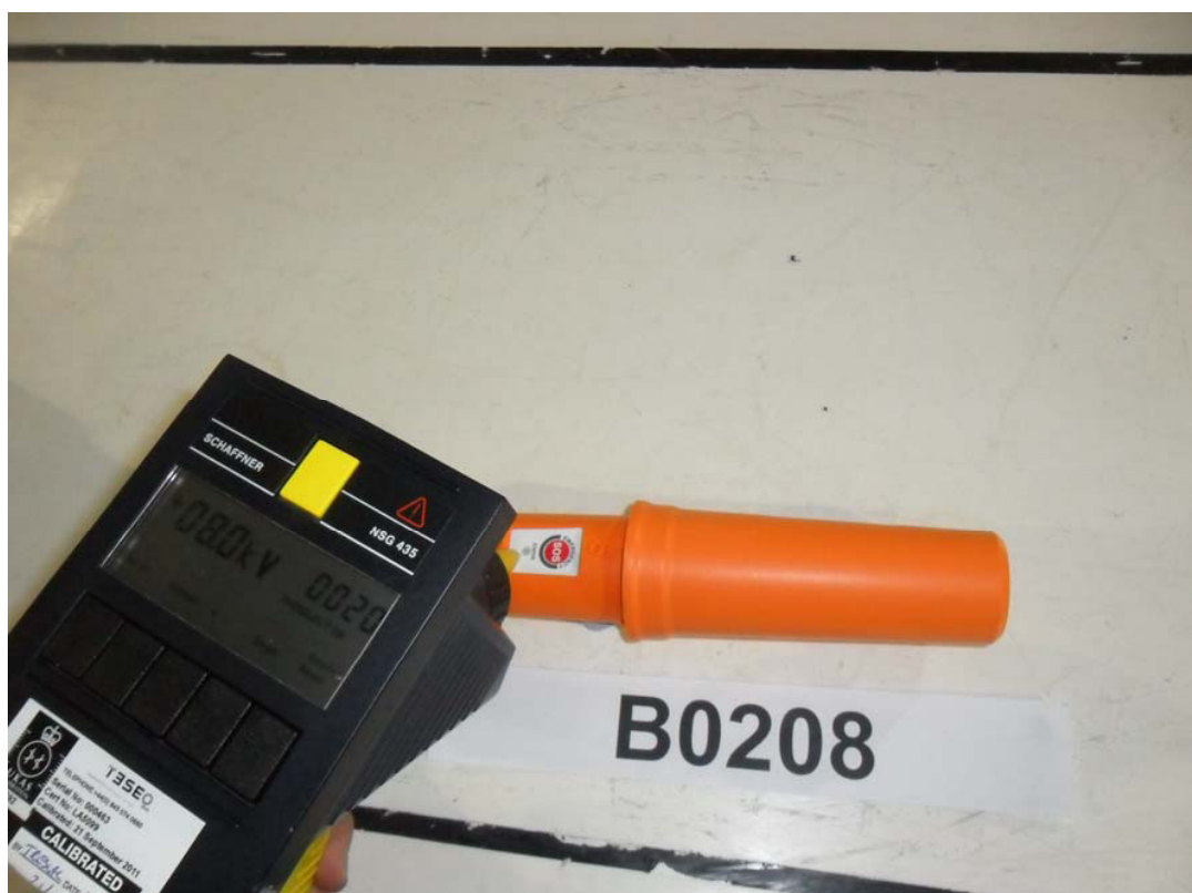
Figure 5.6.4 ESD Testing – Air
