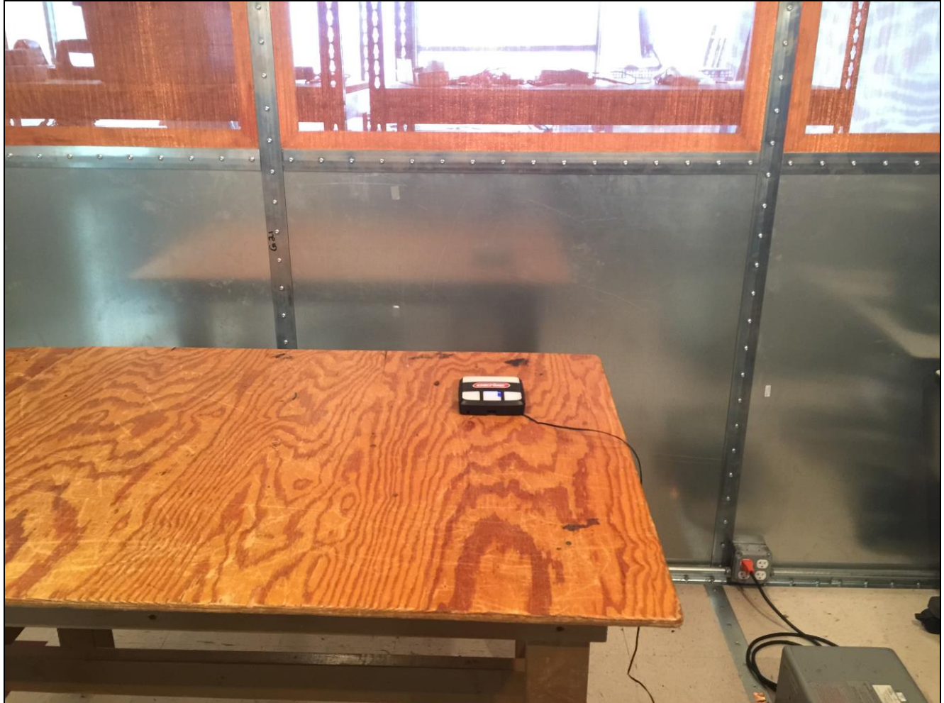
Photograph 3. Conducted Emissions, 15.207(a), Test Setup
