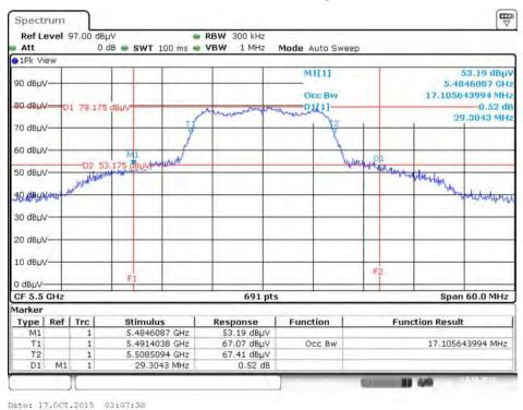
26dB Bandwidth and 99% Occupied Bandwidth Plot on Configuration IEEE 802.11a / Chain 2 / 5580 MHz
