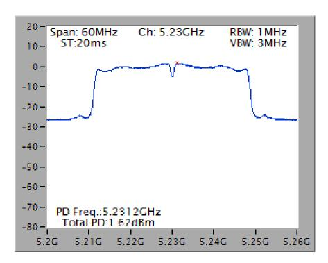
Power Density Plot on Configuration IEEE 802.11n MCS0 HT40 / Chain 1 + Chain 2 / 5270 MHz
