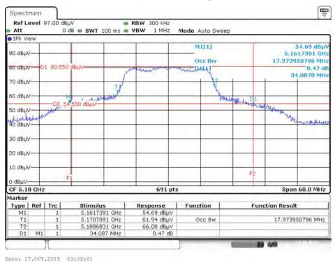
26dB Bandwidth and 99% Occupied Bandwidth Plot on Configuration IEEE 802.11a / Chain 2 / 5200 MHz
