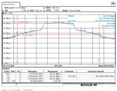
26dB Bandwidth and 99% Occupied Bandwidth Plot on Configuration IEEE 802.11a / Chain 2 / 5320 MHz
