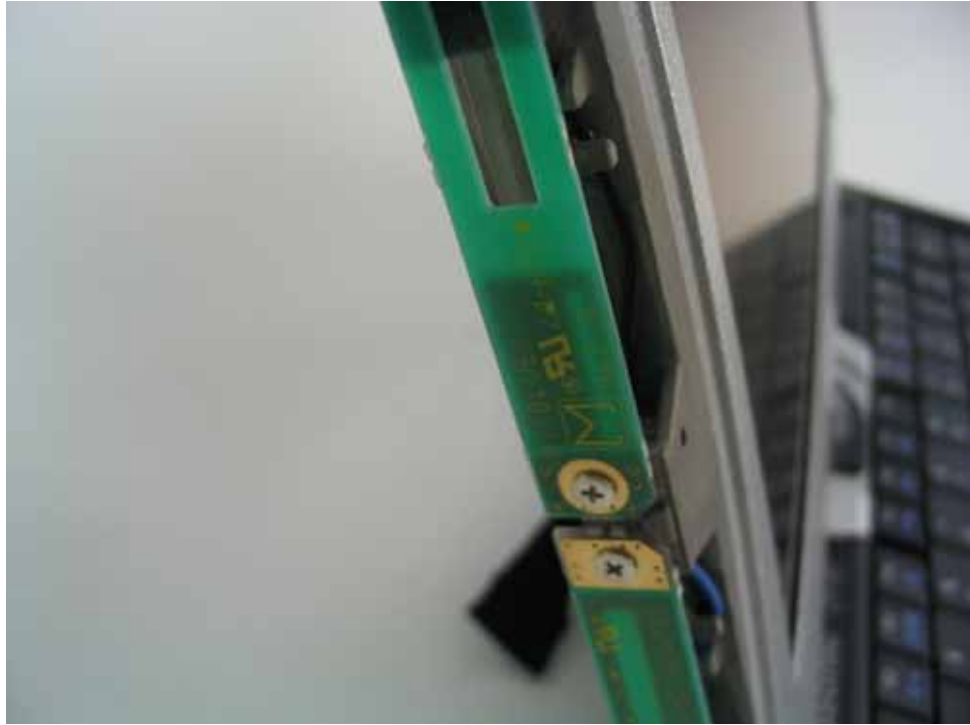
BlueTooth TX/RX Antenna
