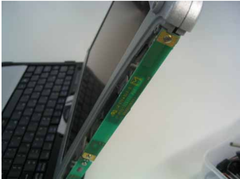
EVDO Main TX/RX Antenna
