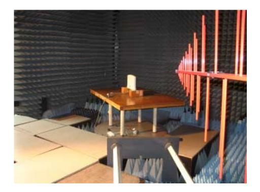
Photograph No.4 Spurious emissions measurement setup in the anechoic chamber above 2900 MHz
