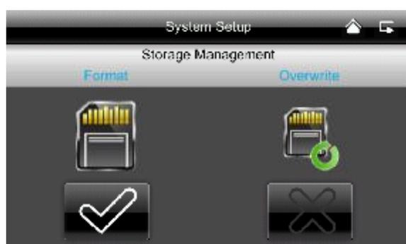
Here you can activate the circular buffer for the recording.
