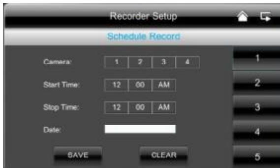
You can save a recording time to start recording at a very specific time.
