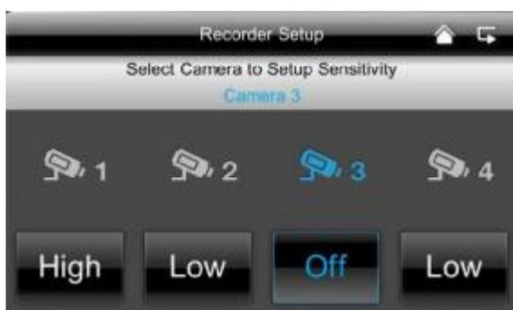
Here you can set the sensitivity of the motion detection for each camera.
