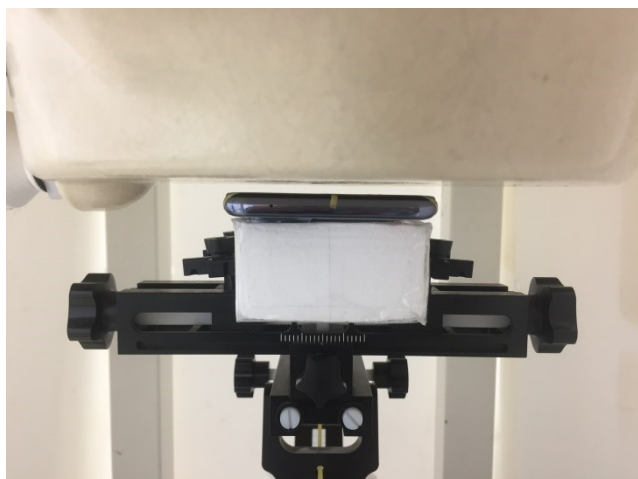
Front, Test Separation 4 mm
