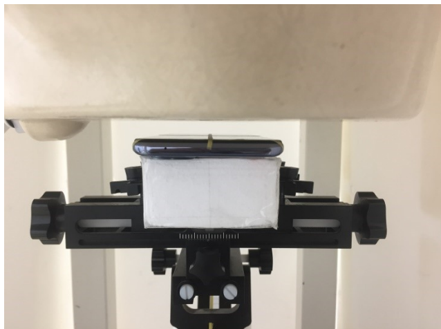
Front, Test Separation 10 mm
