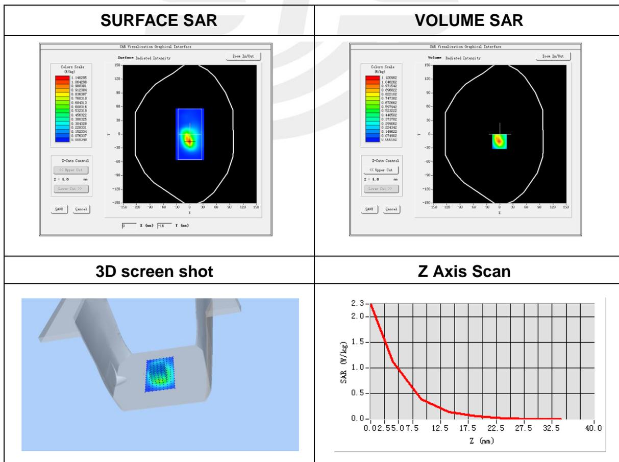
**Plot 3: DUT: GPS Tracker; EUT Model: TRKM010**
