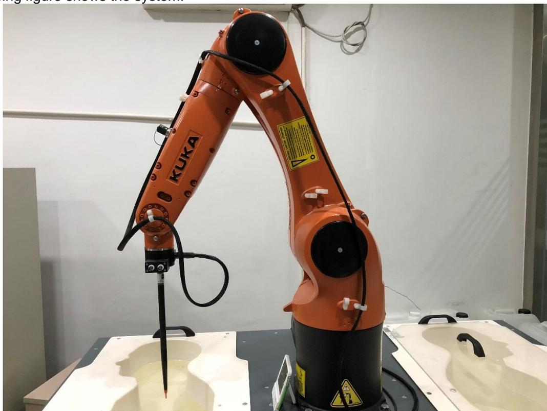
The EUT under test operating at the maximum power level is placed in the phone holder, under the phantom, which is filled with head simulating liquid. The E-Field probe measures the electric field inside the phantom. The Open SAR software computes the results to give a SAR value in a 1g or 10g mass.
