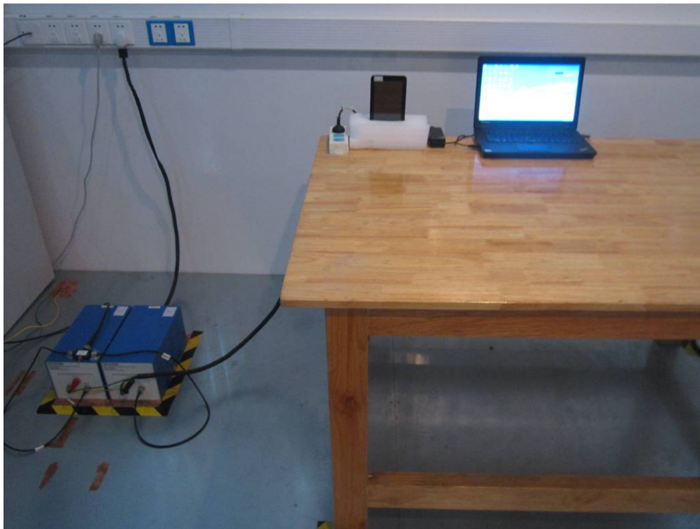
Conducted Emissions Test Setup Front View
