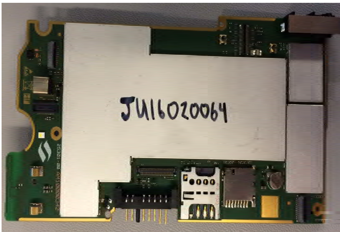
MS2 main PCBA (front) with shields
