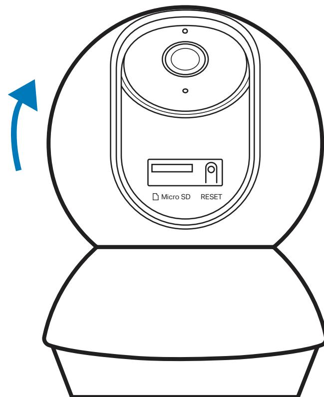
2. Identify the direction of the microSD card and carefully insert the card into the slot. Push in the card until you hear a clicking sound.
