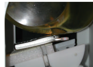
Fig. 18 Head SAR Test Setup
