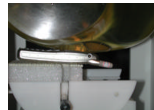
Fig. 20 Head SAR Test Setup
