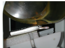
Fig. 15 Head SAR Test Setup
