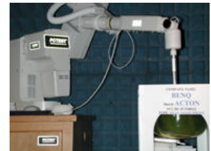
Fig. 1 SAR Test Setup
