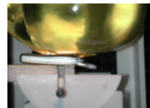
Fig. 21 Head SAR Test Setup
