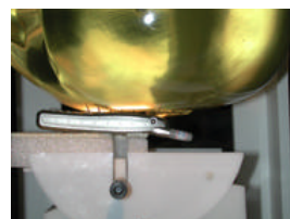
Fig. 16 Head SAR Test Setup
