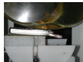
Fig. 17 Head SAR Test Setup
