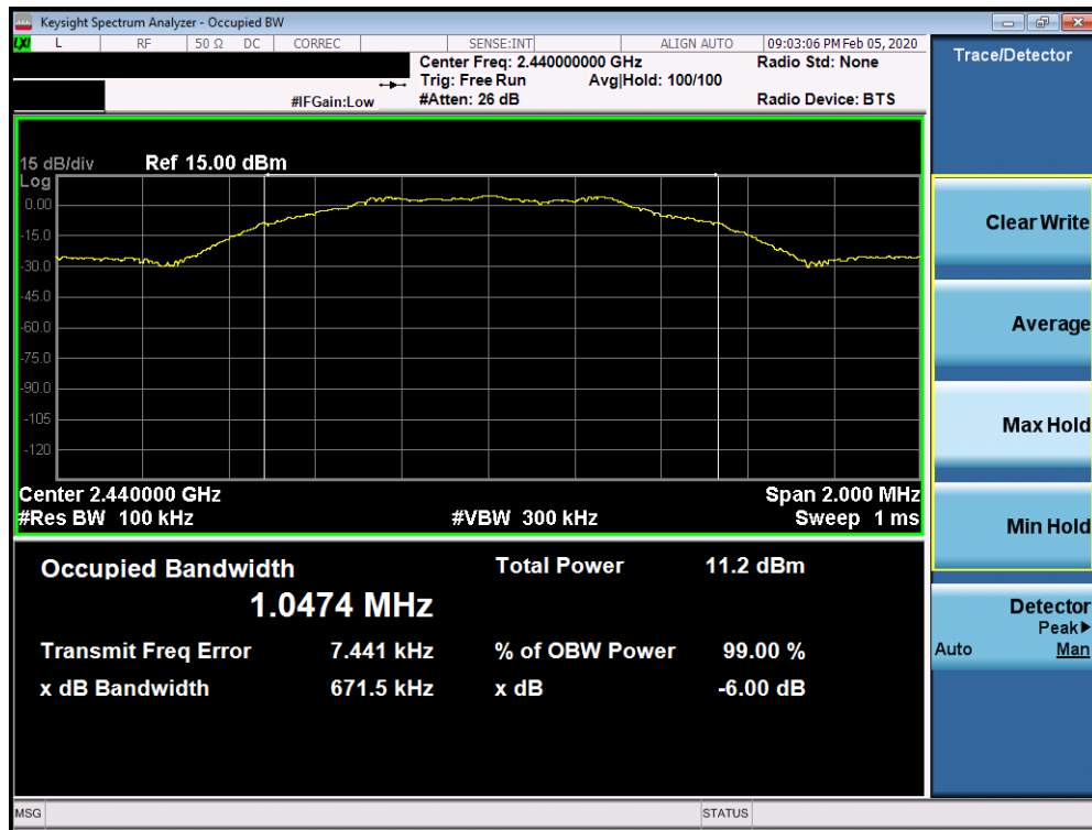
Plot 7-8. 6dB Bandwidth Plot (Bluetooth (LE), 1Mbps – Ch. 19)
