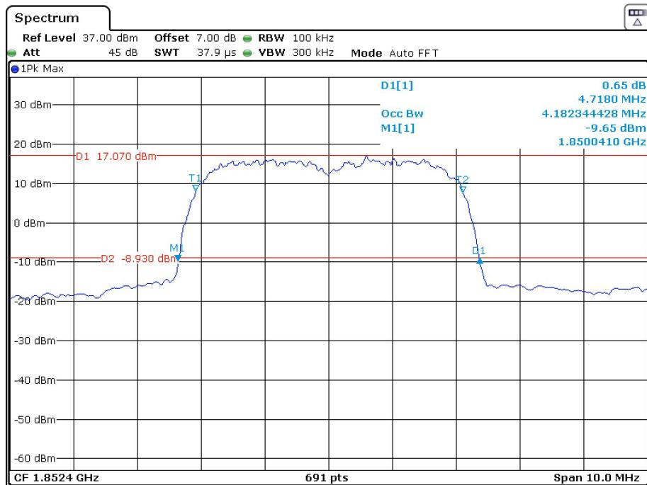
**26 dB Emissions &99% Occupied Bandwidth for HSUPA (QPSK) Mode, Middle channel**
