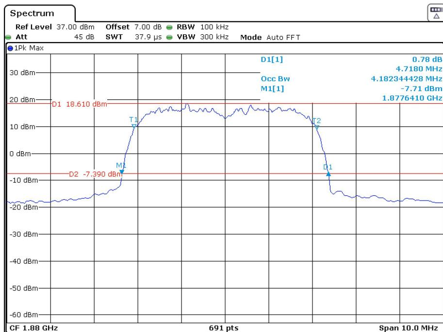
**26 dB Emissions &99% Occupied Bandwidth for HSUPA (QPSK) Mode, High channel**
