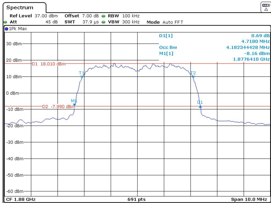
**26 dB Emissions &99% Occupied Bandwidth for HSDPA (16QAM) Mode, High channel**
