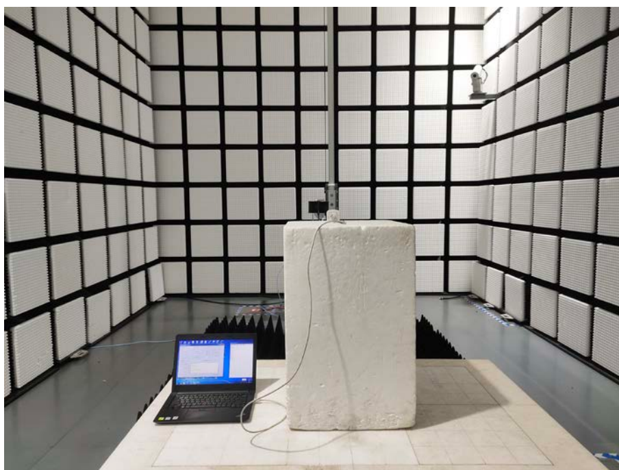
Fig. 3 Radiated emission setup photo(Above 1GHz)
