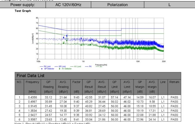
Note: 1. Result (dB $\mu$ V) = Reading (dB $\mu$ V) + Factor (dB).
