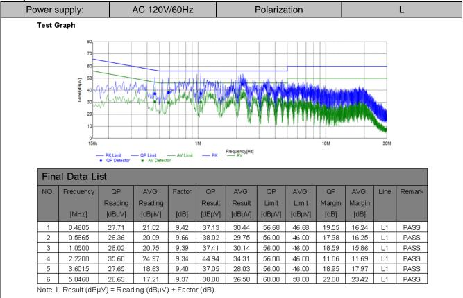
2. Factor (dB) = Cable loss (dB) + LISN Factor (dB).
