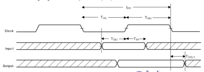
SDIO Protocol Timing Diagram - HighSpeed Mode (3.3V)
