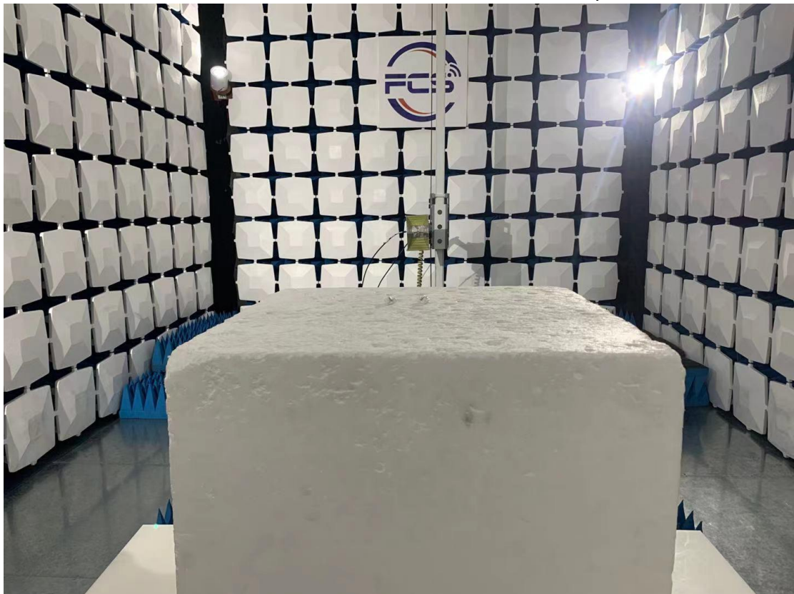
Above 1GHz for radiated emission test setup
