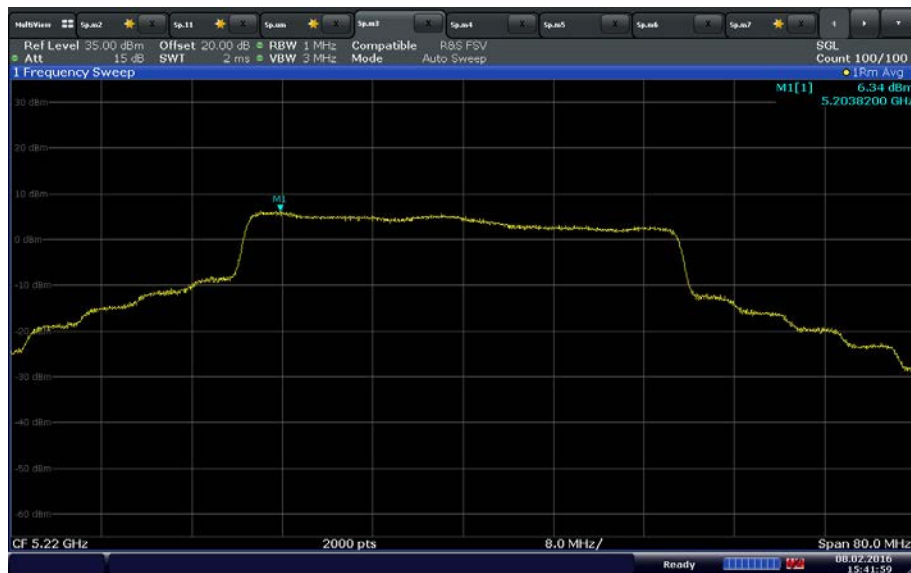
UNII 1 40MHz Bandwidth Mid Channel 5220 MHz
