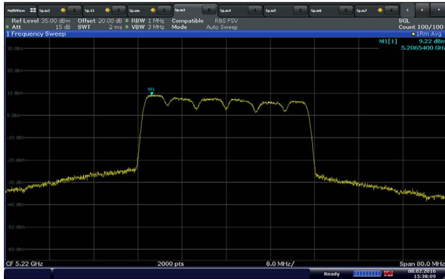
UNII 1 30MHz Bandwidth Middle Channel 5220 MHz
