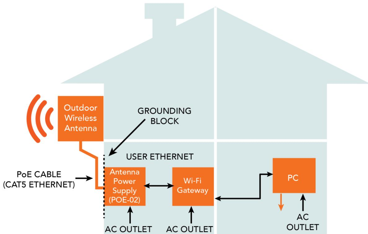
Note that the overall system can have multiple devices that are interconnected via Ethernet cables, and these devices can each have separate connections to the AC outlet and local grounds at different points throughout the home.
