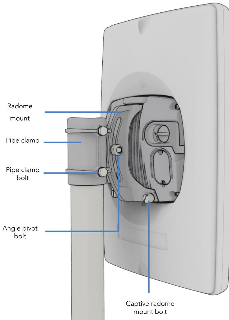
Figure 4 - IFWA-661 mounting bracket and bolts
