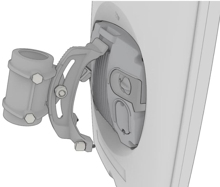
Figure 6 - Attaching the mounting bracket to the Outdoor Wireless Antenna
