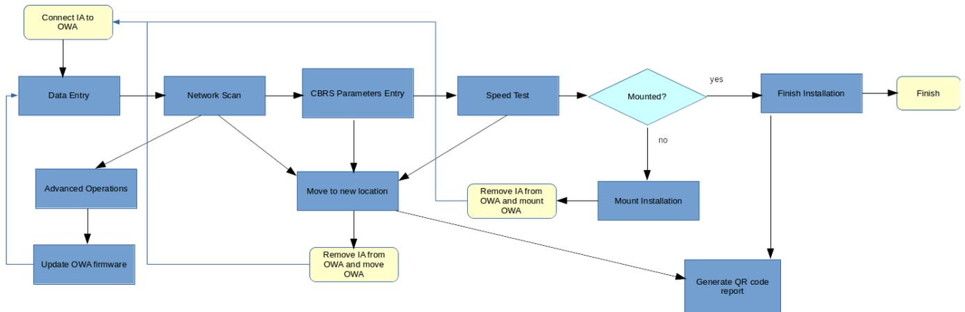
Figure 24 - Alignment process flow
