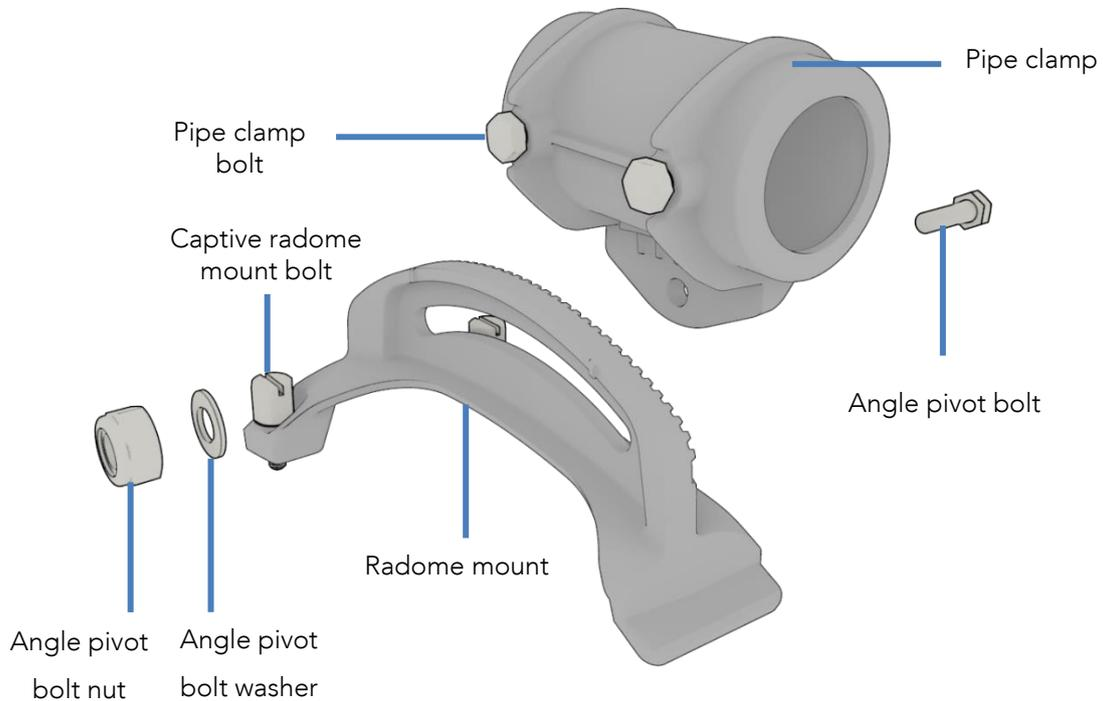
Figure 5 - Mounting bracket assembly
