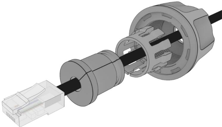
*Figure 17 - Rubber seal placed over Ethernet cable*
