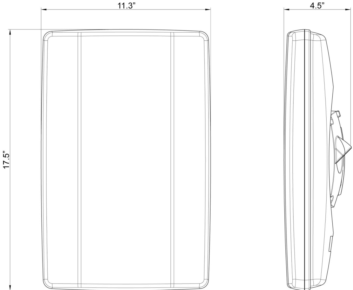
Figure 1 – IFWA-661 Outdoor Wireless Antenna Dimensions
