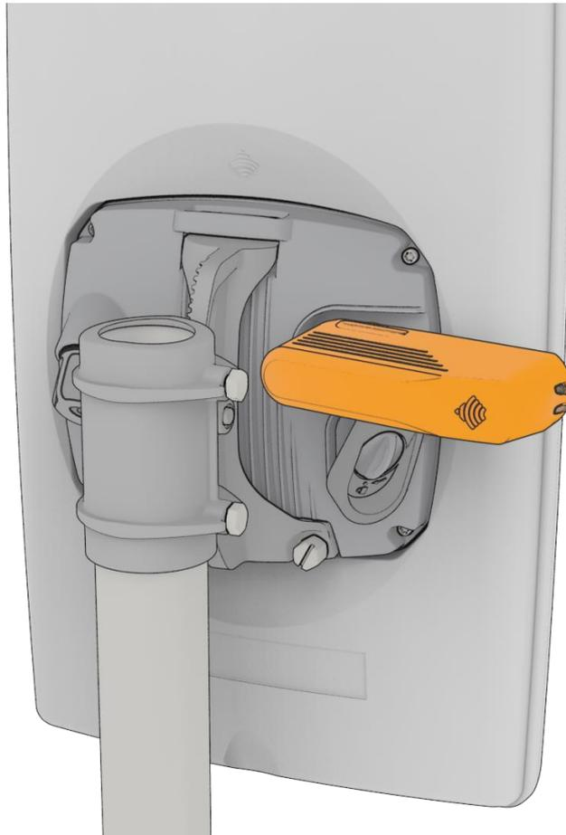
Figure 9 - Attached Smart Antenna Tool
