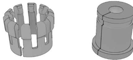
Figure 13 - Rubber seal and ferrule
