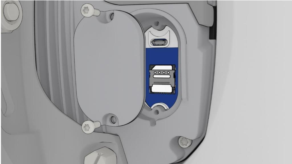
Figure 41 - Replacing the SIM hatch
