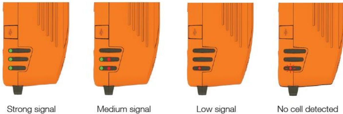
*Figure 10 - Smart Antenna Tool LED statuses in cell scanning mode*
