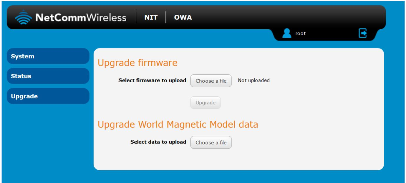
Figure 45 - Smart Antenna Tool firmware and Magnetic Model data upgrade screen
