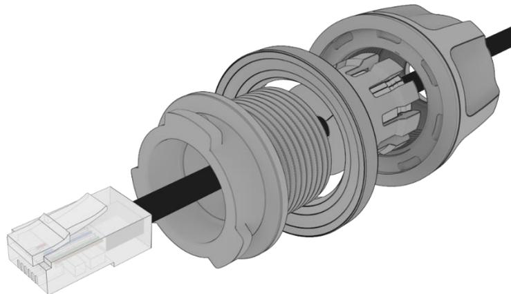
*Figure 20 - Neck placed over Ethernet cable*
