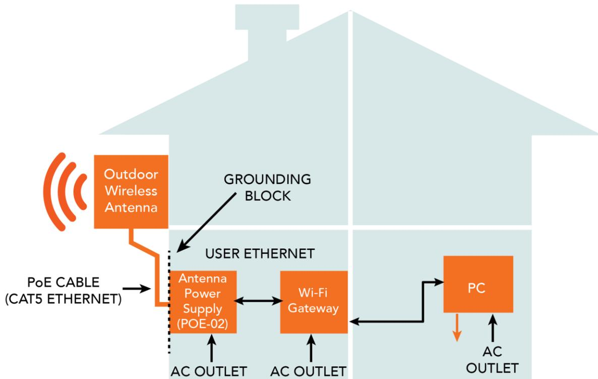
Figure 3 - Typical Outdoor Wireless Antenna Installation
