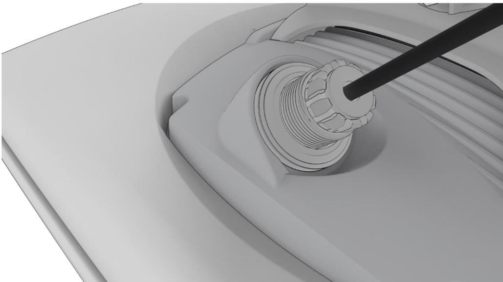
*Figure 22 - Rubber seal and ferrule inserted into neck*
