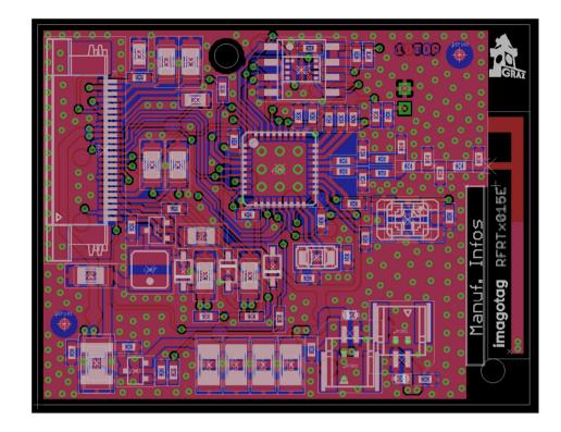
**General changes:** Some parts moved to improve fitting into modified casing. Removing of unnecessary parts. Modified Antenna.
