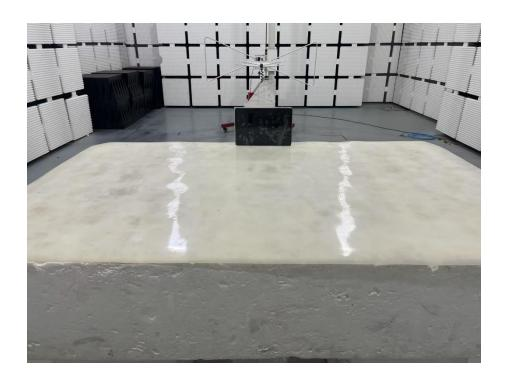
Set-up for Radiated Spurious Emission, Above 1GHz
