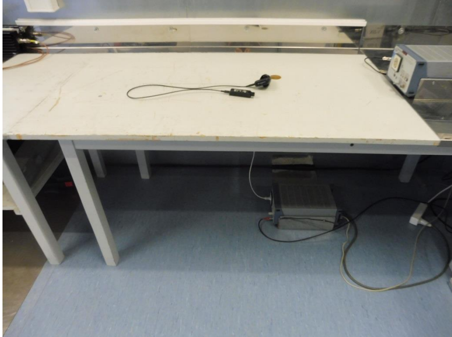
Photo 7: AC conducted test setup
