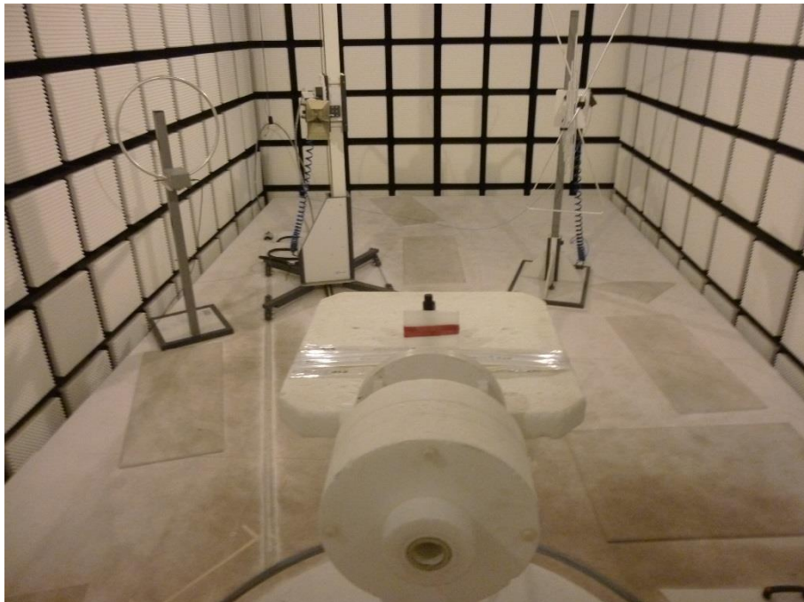
Photo 2: EUT at the anechoic chamber
