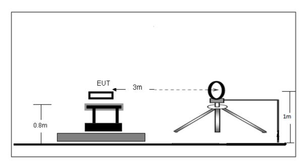
(B) Radiated Emission Test-Up Frequency 30MHz~1GHz
