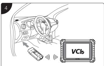
When the MaxiVCI V200 is properly connected to the vehicle and the tablet, the VCI status button on the bottom bar of the screen will display a green badge with a check mark at the corner indicating the tablet is ready to start vehicle diagnosis. A FCC Statement:
