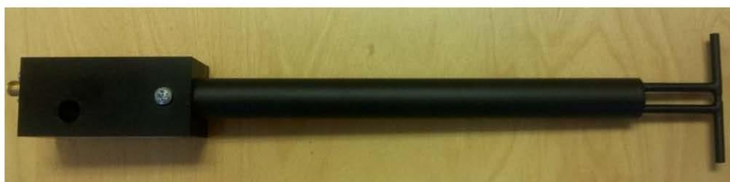
Figure 1 – MVG COMOSAR Validation Dipole
