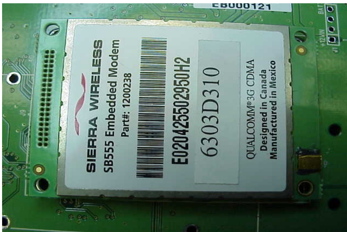
TRANSMITTER, MODEM, TOP SIDE
