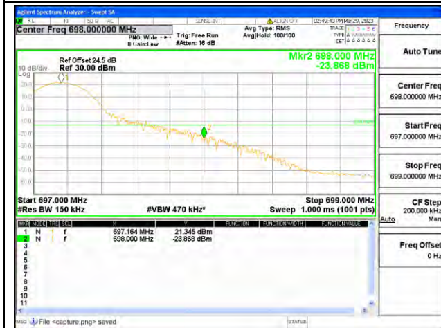
Band71 / 15MHz / High CH / QPSK / 1 RB
