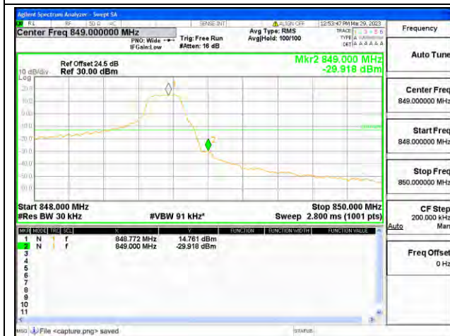
Band5 / 1.4MHz / High CH / QPSK / 1 RB
