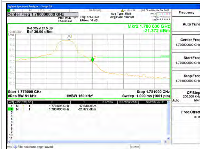
Band66 / 5MHz / High CH / QPSK / 1 RB
