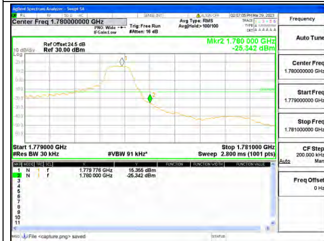
Band66 / 1.4MHz / High CH / QPSK / 1 RB
