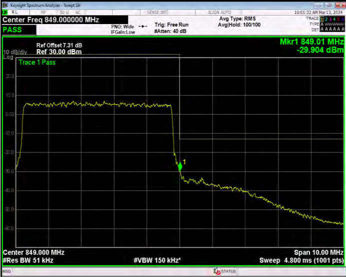
Band66 16QAM BW=1.4MHz Channel=131979 RB Size=1 Position=#0
