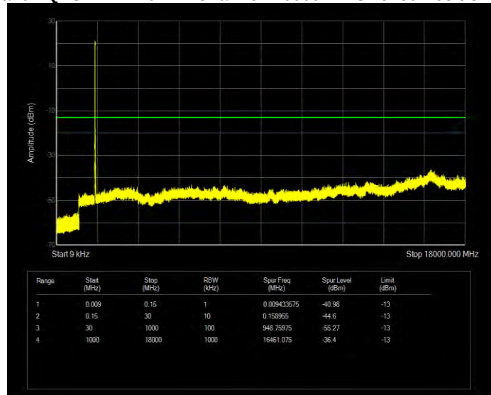
Band4 QPSK BW=10MHz Channel=20175 RB Size=50 Position=#0
