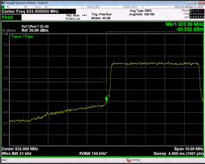
Band26(824-849) QPSK BW=5MHz Channel=27015 RB Size=25 Position=#0
