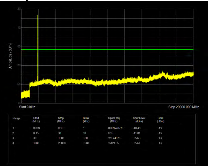
Band2 16QAM BW=1.4MHz Channel=19193 RB Size=6 Position=#0
