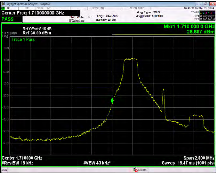
Band66 16QAM BW=1.4MHz Channel=131979 RB Size=1 Position=#0
