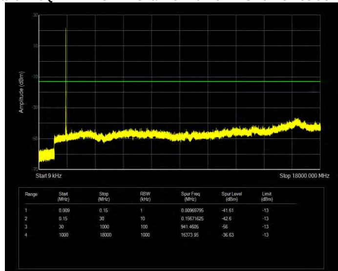
Band4 16QAM BW=3MHz Channel=20385 RB Size=15 Position=#0
