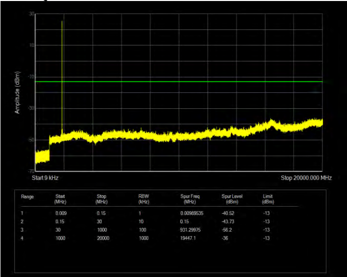
Band2 16QAM BW=1.4MHz Channel=19193 RB Size=6 Position=#0
