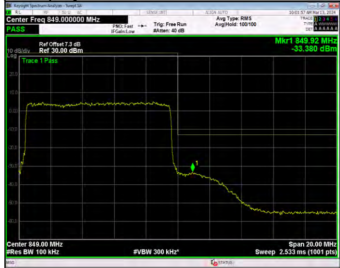
Band26(824-849) 16QAM BW=15MHz Channel=26865 RB Size=75 Position=#0
