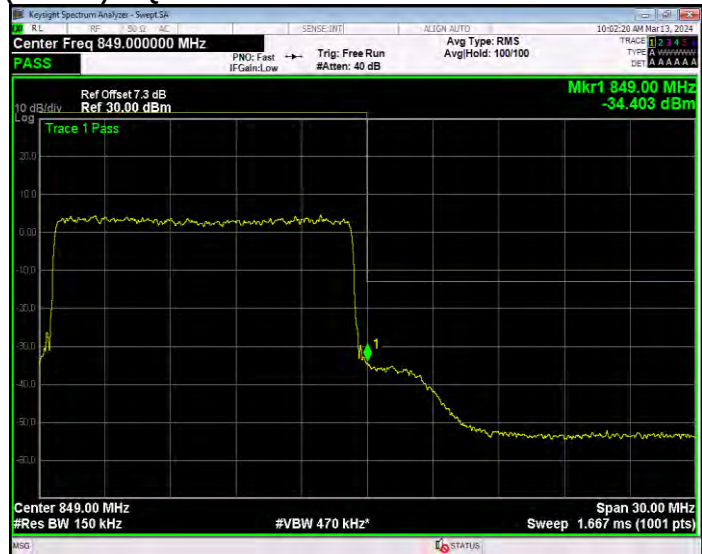
Band26(824-849) 16QAM BW=15MHz Channel=26965 RB Size=75 Position=#0
