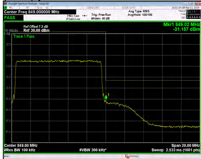
Band26(824-849) QPSK BW=15MHz Channel=26865 RB Size=75 Position=#0
