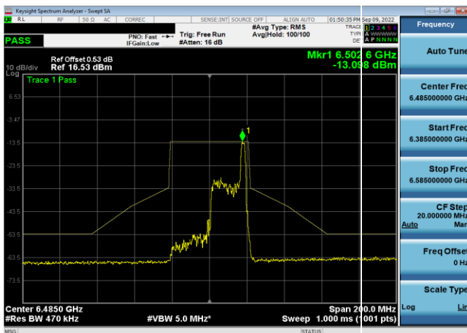
Plot 7-556. In-Band Emission Plot SDM Antenna WF5t (40MHz 802.11ax RU26 (UNII Band 6) – Ch. 107)
