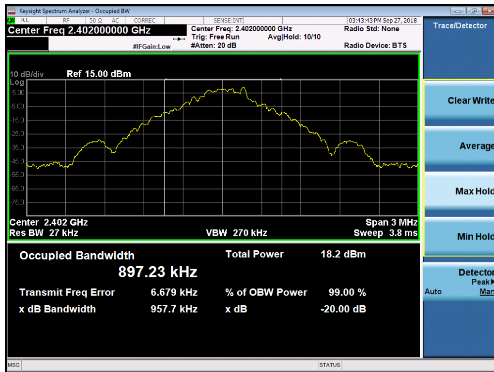
Plot 7-1. 20dB Bandwidth Plot (Bluetooth, 1Mbps – Ch. 0)
