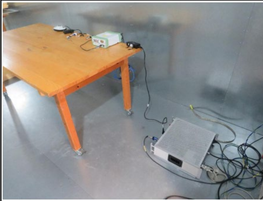
Setup for measurements 150 kHz – 30 MHz (with PoE)
