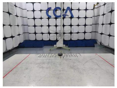
Radiated emission Test Setup (Above 1GHz)
