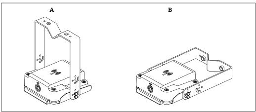
Installation with "Mounting bracket wall/ceiling".
