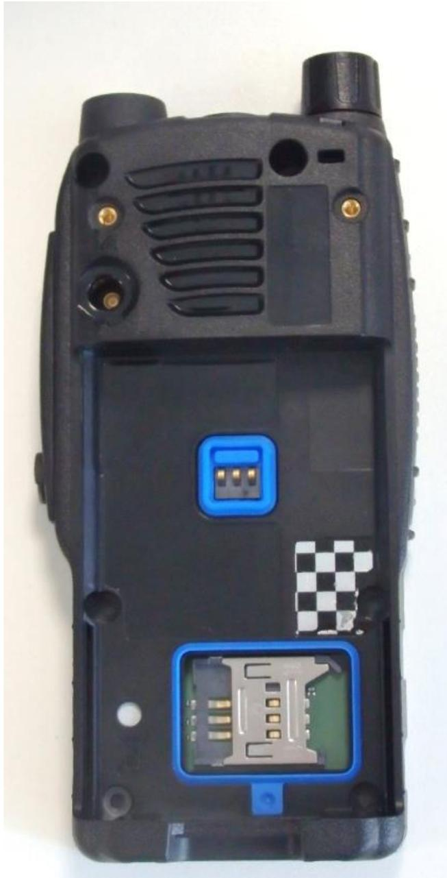
Figure 4. SC21 Series Top with Battery and Antenna Removed
