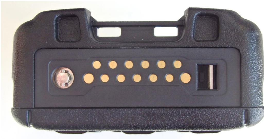
Figure 6. SC21 Series PTT Side with Battery and Antenna Removed
