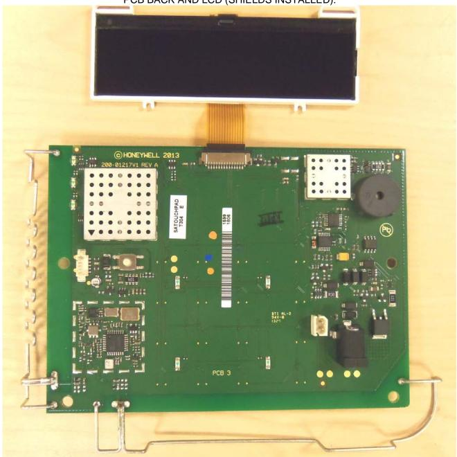
Note - of the three shields, the lower left shield is never populated on this assembly.
