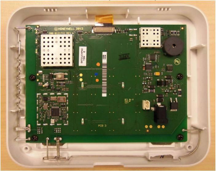
Note - of the three shields, the lower left shield is never populated on this assembly.
