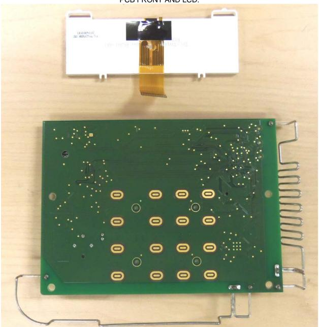
PCB BACK AND LCD (SHIELDS INSTALLED):
