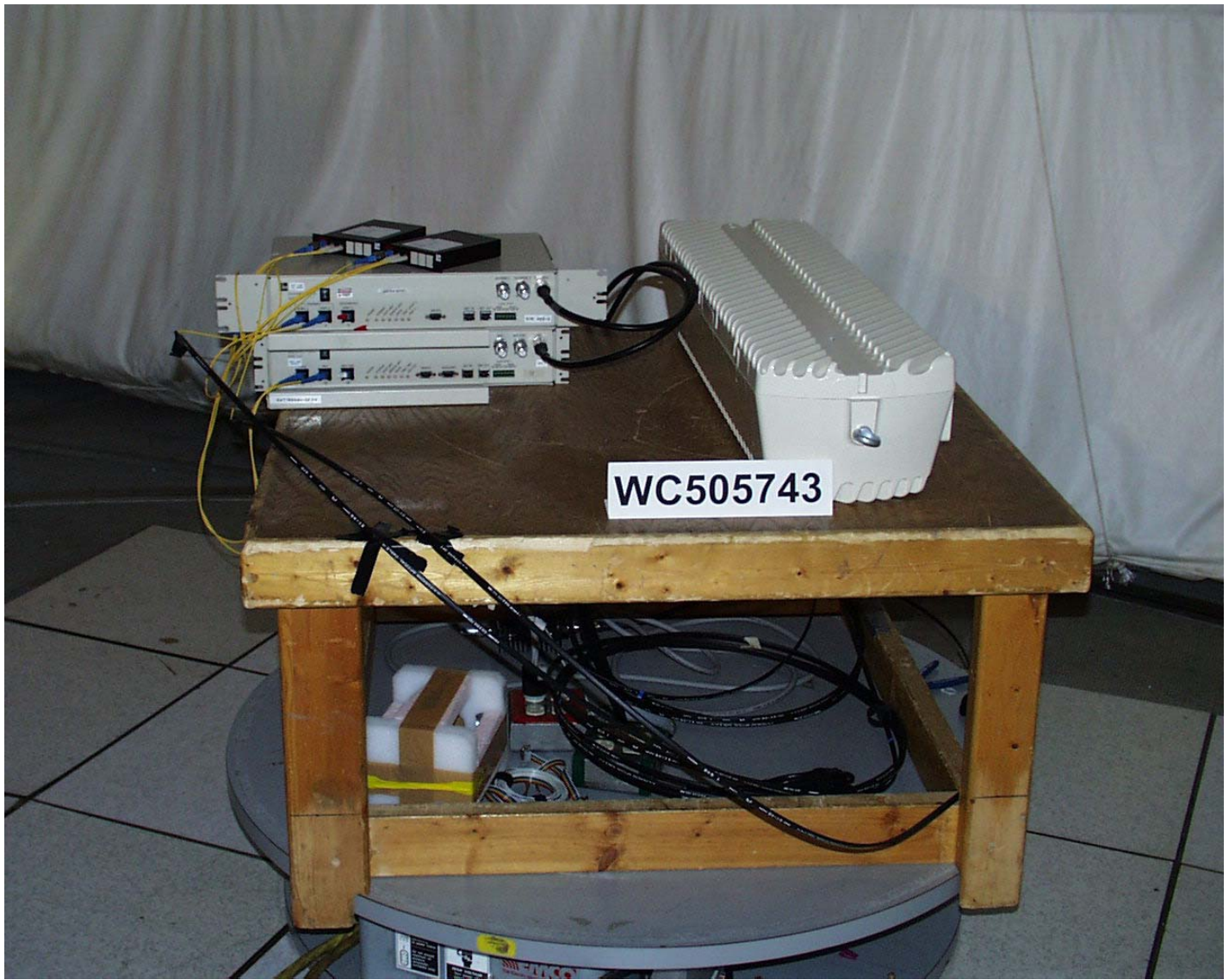
Test setup photo, radiated emissions
