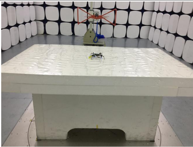
Radiated Spurious Emissions Test Setup Below 1GHz
