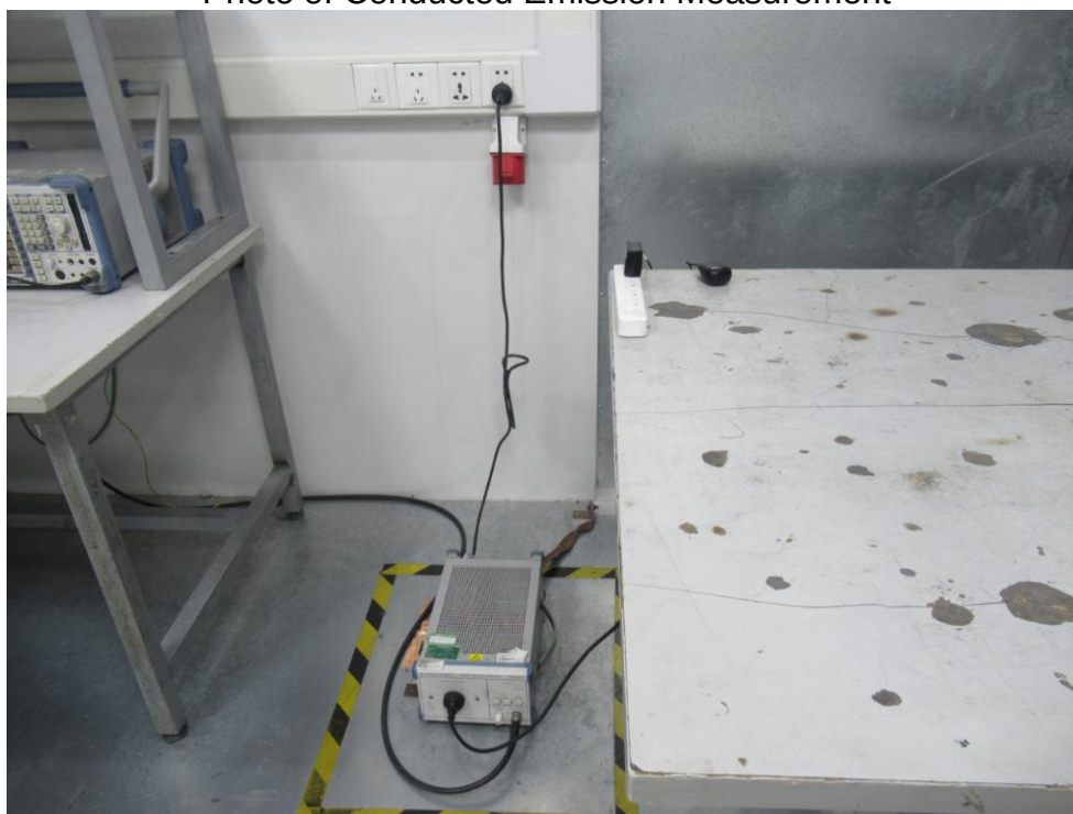
FCC ID: 2AMPLNE-980 Photo of Conducted Emission Measurement
