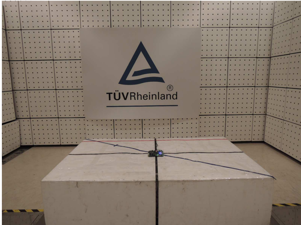
Photograph 1: Set-up for Spurious Emissions (Front View)
