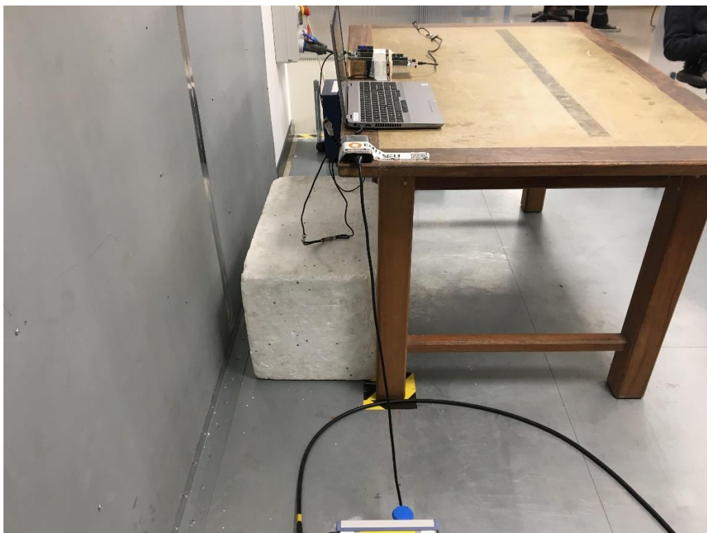
TEST SETUP PHOTO(S) - 120VAC/60Hz POWER SUPPLY / CARD EMULATION MODE
