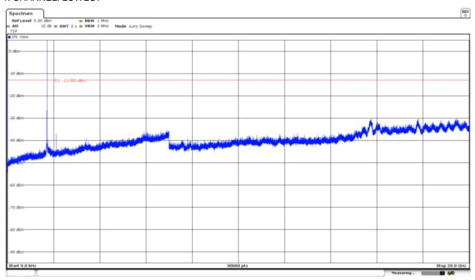
Note: The peak above the limit is the carrier frequency. The peak at 1805MHz corresponds to the downlink signal.
