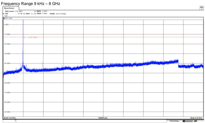
Note: The peak above the limit is the carrier frequency. The peak at 746MHz corresponds to the downlink signal.
