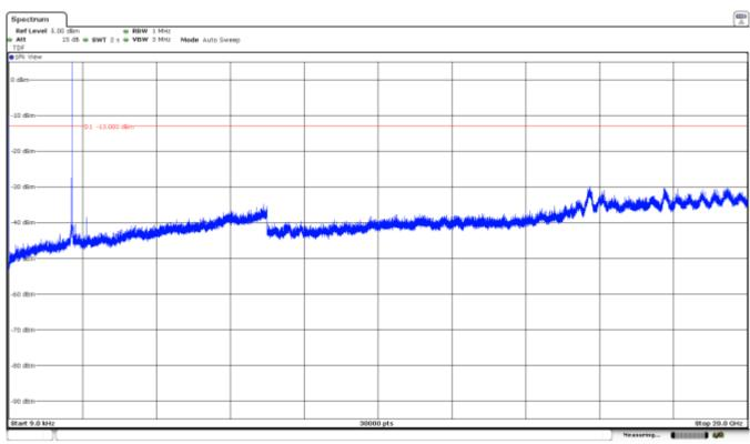
Note: The peak above the limit is the carrier frequency. The peak at 1805MHz corresponds to the downlink signal.
