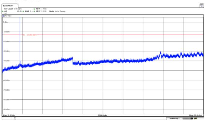
Note: The peak above the limit is the carrier frequency. The peak at 1840MHz corresponds to the downlink signal.
