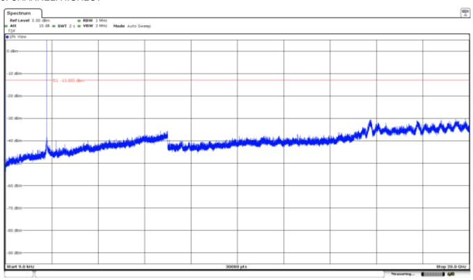
Note: The peak above the limit is the carrier frequency. The peak at 1875MHz corresponds to the downlink signal.
