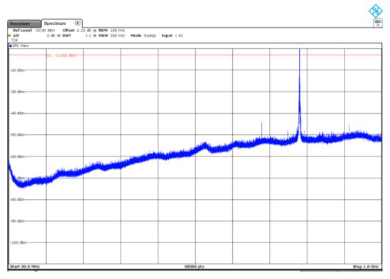
Note: The peak above the limit is the carrier frequency. The peak at 756MHz corresponds to the downlink signal.
