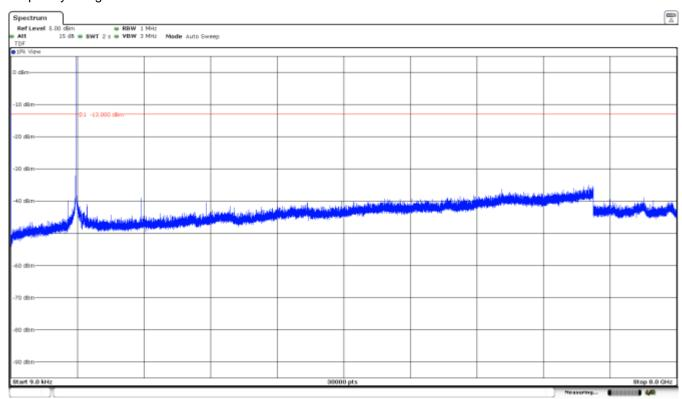
Note: The peak above the limit is the carrier frequency. The peak at 751MHz corresponds to the downlink signal.
