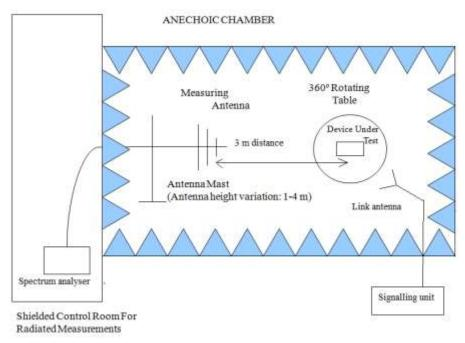
Radiated measurements above 1 GHz.
