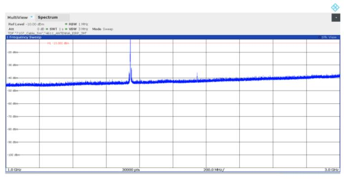
Note: The peak above the limit is the carrier frequency. The peak at 2145MHz corresponds to the downlink signal.
