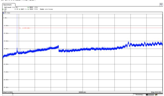
Note: The peak above the limit is the carrier frequency. The peak at 1875MHz corresponds to the downlink signal.
