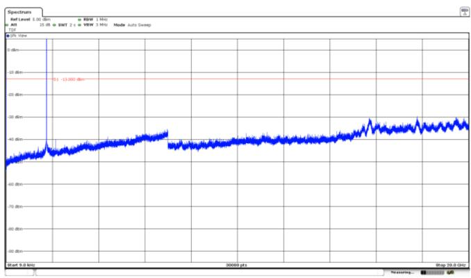
Note: The peak above the limit is the carrier frequency. The peak at 1840MHz corresponds to the downlink signal.
