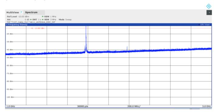
Note: The peak above the limit is the carrier frequency. The peak at 2179.8MHz corresponds to the downlink signal.
