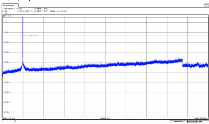
Note: The peak above the limit is the carrier frequency. The peak at 756MHz corresponds to the downlink signal.
