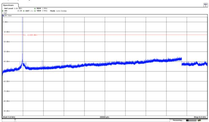
Note: The peak above the limit is the carrier frequency. The peak at 746MHz corresponds to the downlink signal.
