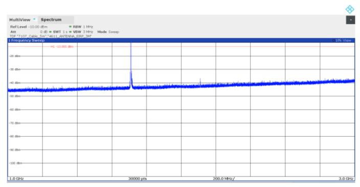
Note: The peak above the limit is the carrier frequency. The peak at 2110.2MHz corresponds to the downlink signal.
