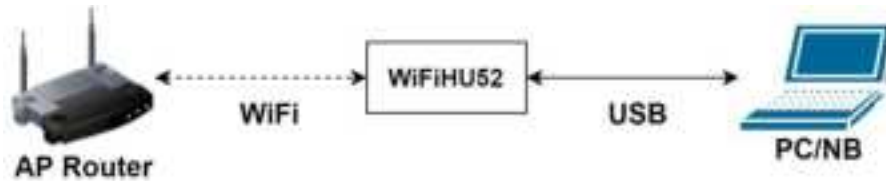
Figure 46 Test WiFi environment under Ubuntu 16.04 Linux
